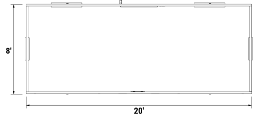
COLLAPSIBLE MODULAR UNIT TOP VIEW
